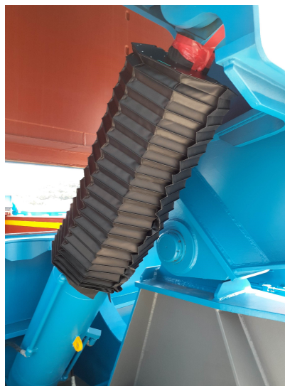
Photo 3) Bellow cover of the hydraulic cylinder for end-folding type hatch cover (developing)
