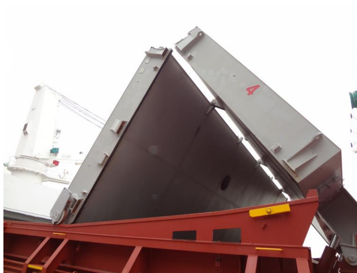
Photo 1) Hatch cover partial opening
